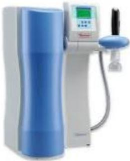
*Barnstead GenPure PRO offers outstanding control, high-precision, and USP-complying conductivity measurement with temperature compensation that can be switched on or off. The Barnstead GenPure system delivers ultrapure 18.2MW.cm water with consistent quality for the most demanding and sensitive applications.*
