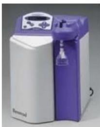
The most complete water system on the market today. Includes the latest advances in ion exchange and filtration technologies as well as a dual wavelength UV lamp and ultrafilter. Multi-language display.
